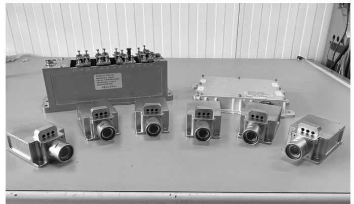
VIKI – Integrated Independent Video Kit for use on the Ariane 6 launch vehicle
