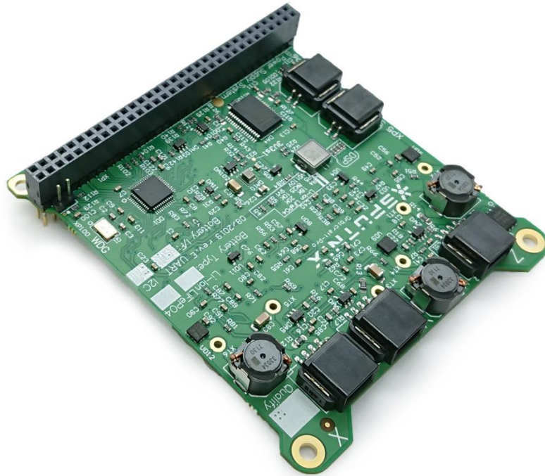
Figure 7. OrbiCraft-Pro power supply unit.
