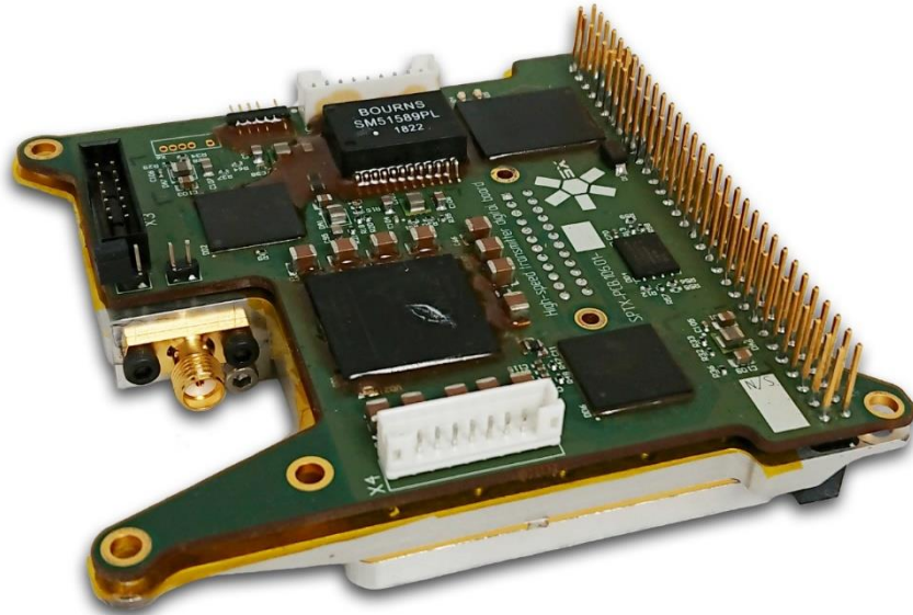
Figure 23. OrbiCraft-Pro X-band transmitter.
