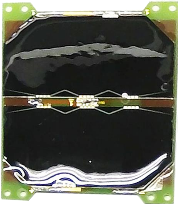
Figure 12. OrbiCraft-Pro GaAs side solar panel with coils.
