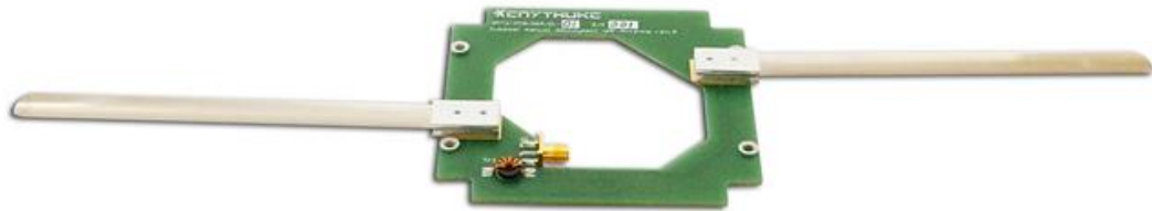
Figure 9. OrbiCraft-Pro UHF antenna system.
